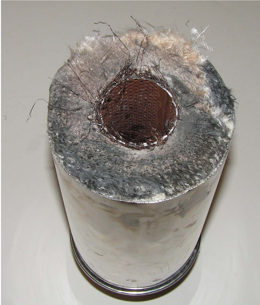
Figure 3.4 (b) The Type 20 muffler, cut away view.
